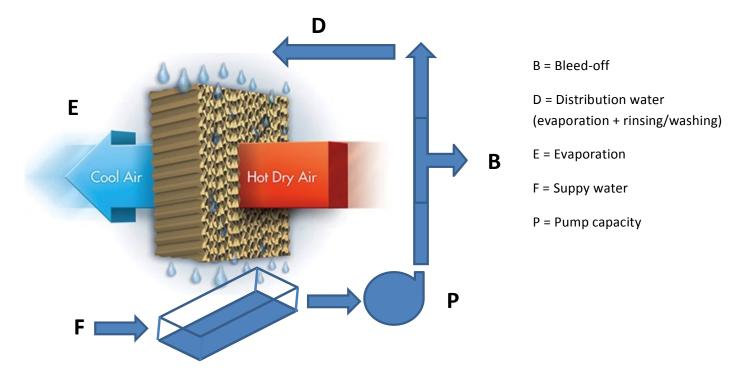
$$P(pump capacity) = D(distribution) + B(bleed-off)$$
