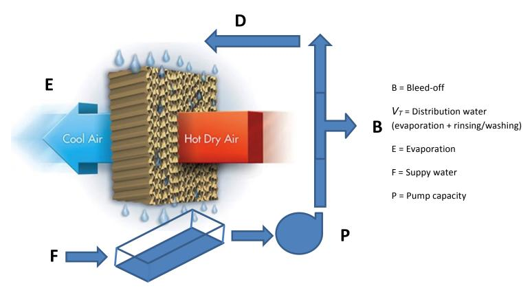
$P(pump \ capacity) = V_T(distribution \ water) + B(bleed-off)$
