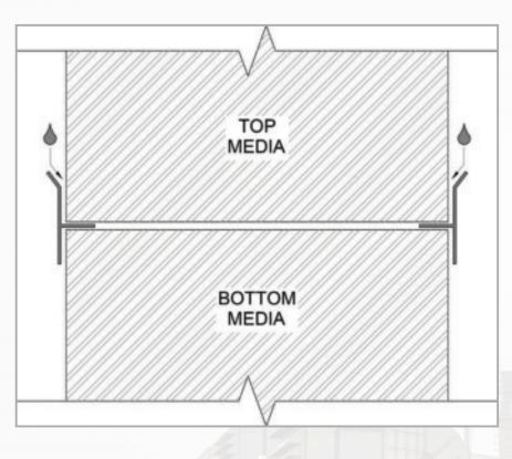
Vertical T-bars for vertical joints where media is inserted where a vertical gap could be present after installation. If a bank should be greater than 120" (3m) in height, then two separate systems need to be installed on top of each other. For the reasons above, two separate systems - top-supply and bottom-drain configurations - must be used.
