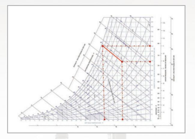
Using a psychrometric chart to find the absolute humidity of the air entry and the T<sub>leaving</sub>, in lb<sub>w</sub>/lb<sub>dry air</sub>, then the amount of water absorbed by the air can be calculated using the following formula;
