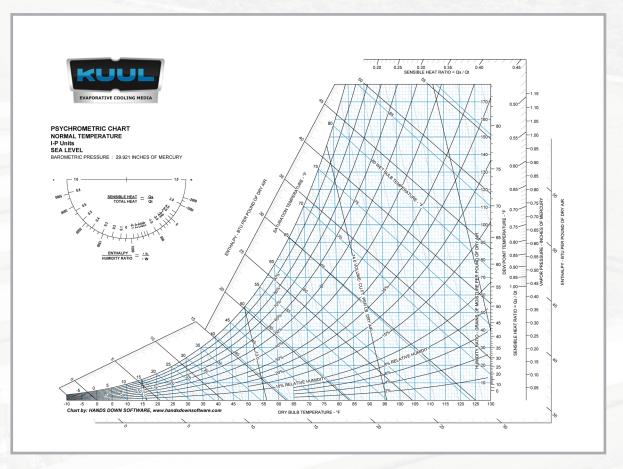
• Using a psychrometric chart to find the absolute humidity of the air entry and the Tleaving, in lbw/lbdryair, then the amount of water absorbed by the air can be calculated using the following formula;
