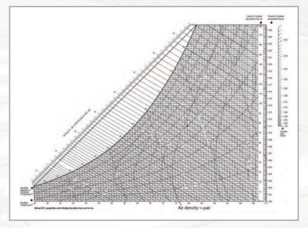
• Using a psychrometric chart to find the absolute humidity of the air entry and the Tleaving, in Ibw/Ibdryair, then the amount of water absorbed by the air can be calculated using the following formula;
