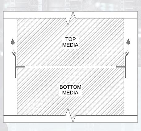
Vertical T-bars for vertical joints where media is inserted where a vertical gap could be present after installation. If a bank should be greater than 100" (2.54m) in height, then two separate systems need to be installed on top of each other. For the reasons above, two separate systems (top-supply and bottom-drain configurations) must be used.
