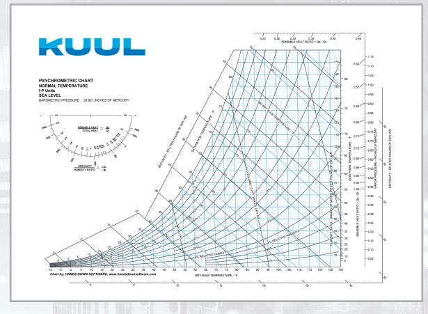
• Using a psychrometric chart to find the absolute humidity of the air entry and the T<sub>leaving</sub>, in lb<sub>w</sub>/lb<sub>dry air</sub>, then the amount of water absorbed by the air can be calculated using the following formula;
